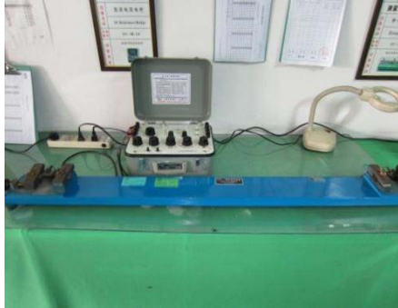
DC Resistance Bridge
